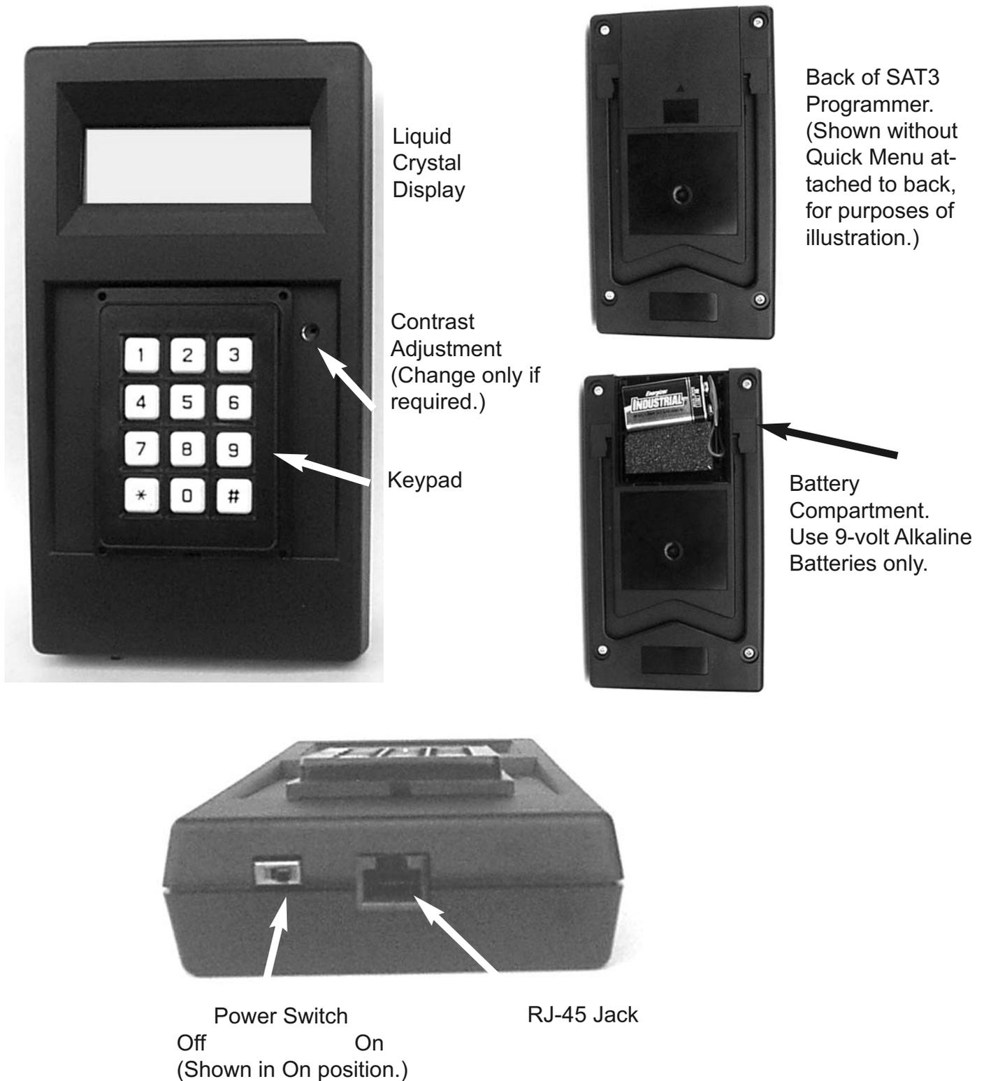
**WARNING:** RJ-45 connector is NOT a standard Ethernet connection. Do NOT plug either SAT3 or SAT3 Programmer into an Ethernet jack on laptop or computer. You WILL damage the SAT3 and the SAT3 Programmer.
