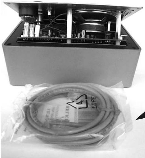
Remove the supplied RJ-45 7-foot CAT5e patch cable from its package and connect one end to the SAT3 RJ-45 jack.
